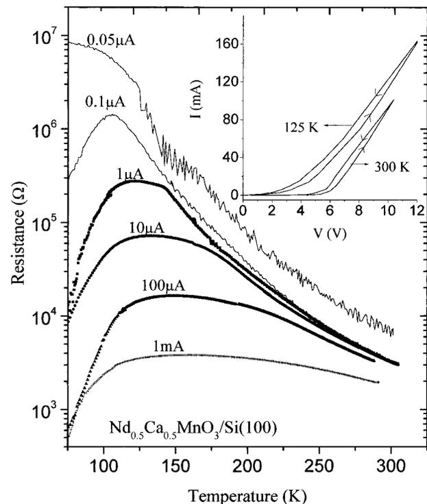
FIG. 1. Temperature variation of the resistance of a polycrystalline  $\text{Nd}_{0.5}\text{Ca}_{0.5}\text{MnO}_3$  film deposited on Si(100) for different values of current. Inset shows  $I$ – $V$  characteristics at two temperatures.
