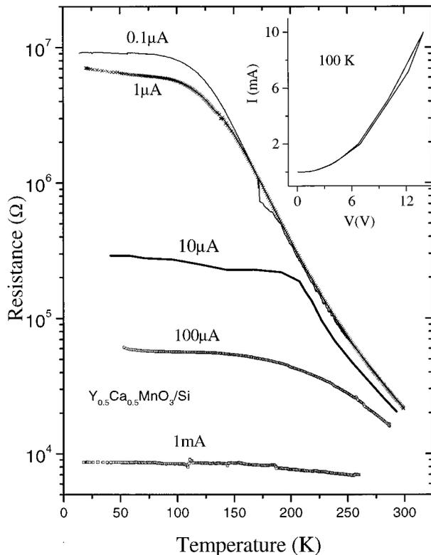
FIG. 3. Temperature variation of the resistance of a polycrystalline  $\text{Y}_{0.5}\text{Ca}_{0.5}\text{MnO}_3$  film deposited on  $\text{Si}(100)$  for different values of current. Inset shows  $I-V$  characteristics at 100 K.
