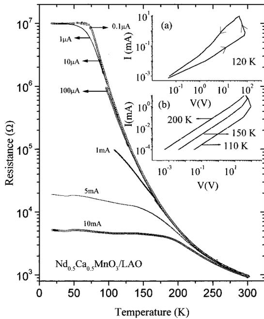
FIG. 2. Temperature variation of the resistance of an oriented  $\text{Nd}_{0.5}\text{Ca}_{0.5}\text{MnO}_3$  film deposited on  $\text{LaAlO}_3(100)$  for different values of current. Insets show  $I-V$  curves demonstrating (a) hysteresis and (b) non-ohmic behavior.
