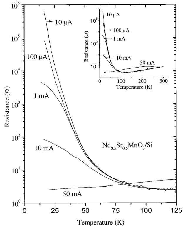
FIG. 4. Temperature variation of the resistance of a polycrystalline  $\text{Nd}_{0.5}\text{Sr}_{0.5}\text{MnO}_3$  film deposited on  $\text{Si}(100)$  for different values of current. Inset shows data over a wide temperature range.
