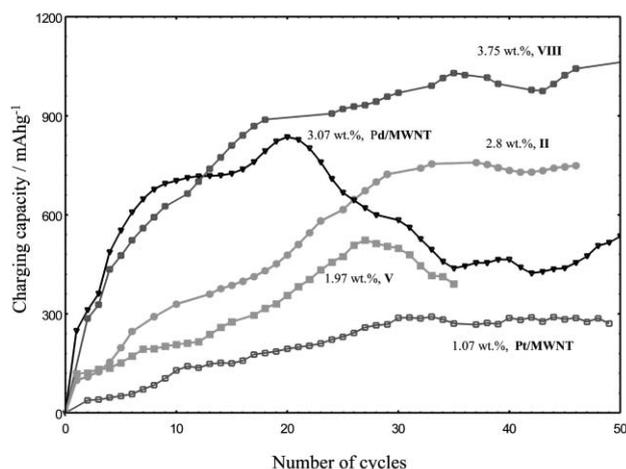
Fig. 7 Plot of the charging capacity against the number of cycles for different carbon nanostructures. Also shown are the corresponding weight percentages of H<sub>2</sub> stored.
